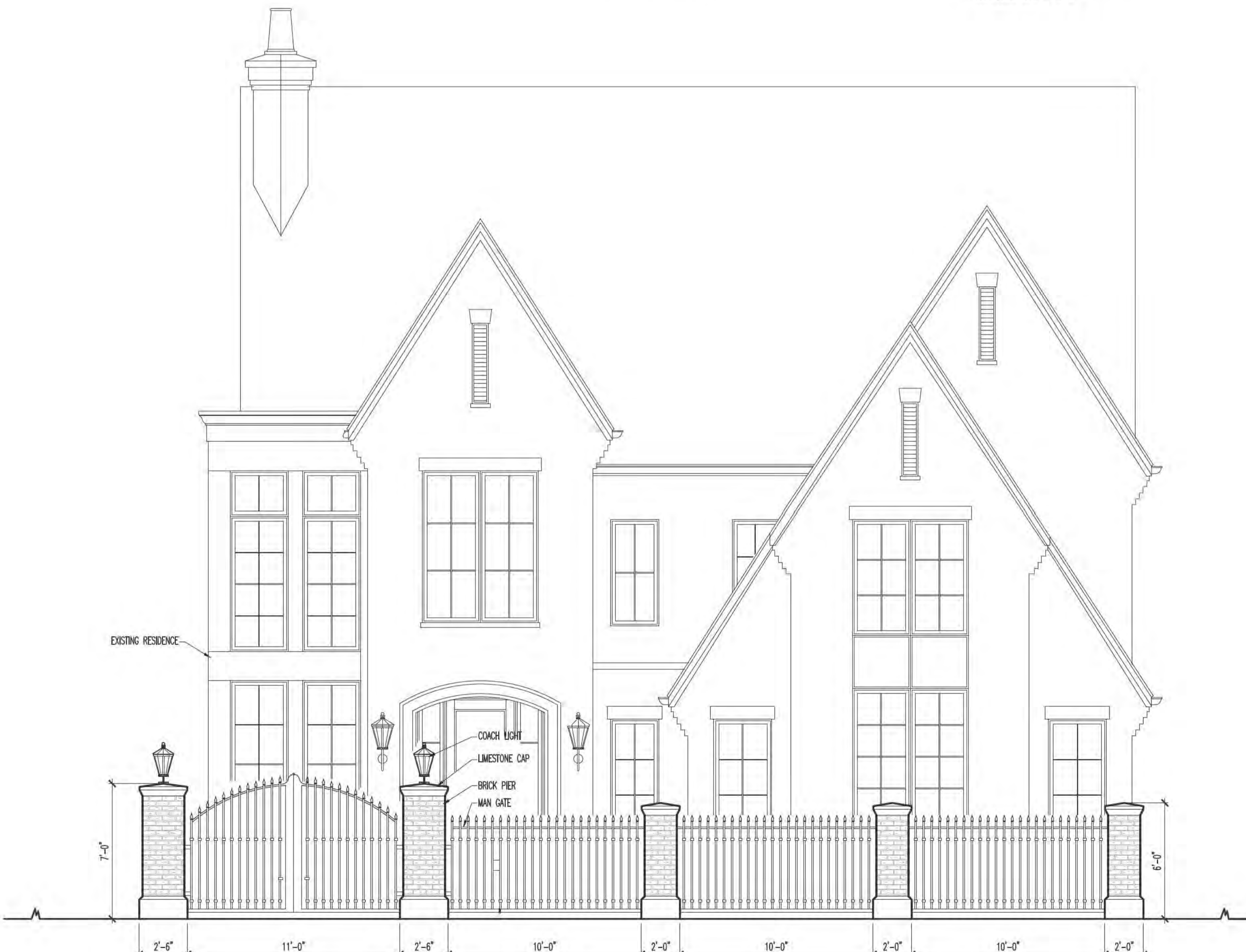
FENCE ELEVATION @ STREET SCALE: 1/4" = 1'-0"
