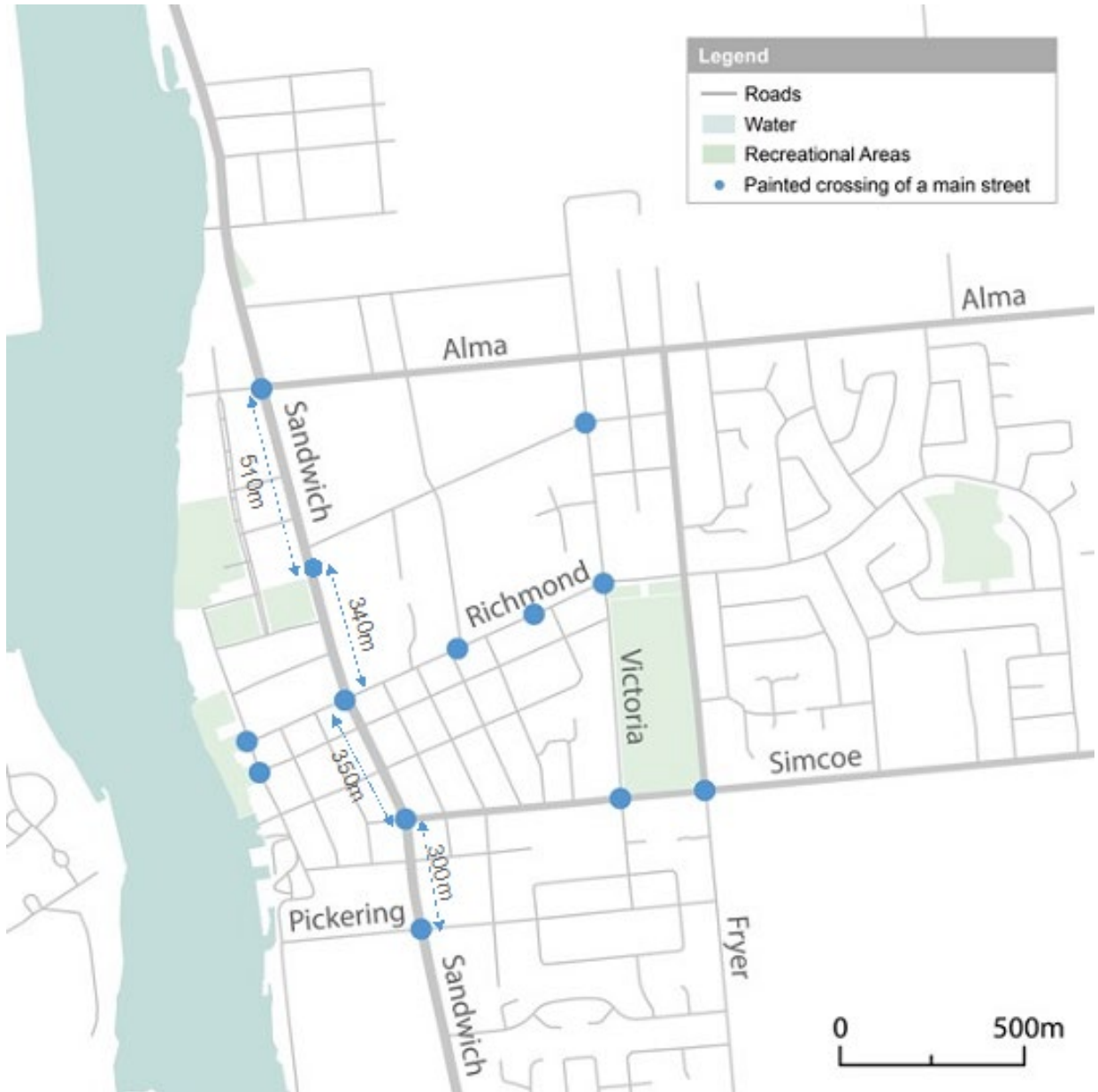
Figure 4-22: Distance between Formal Crossing Locations along Sandwich Street
