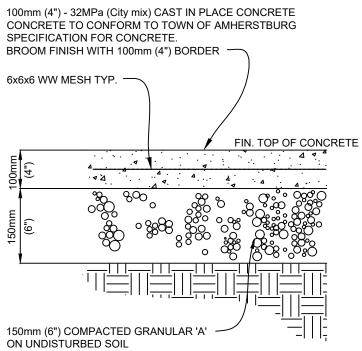
PROVIDE SAWCUT CONTROL JOINTS (40mm DEEP) AT APPROXIMATELY 2.0m O.C.
